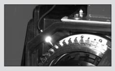
The fact that many non-magnetic metals allow magnetic fields to pass unhindered also extends the fields of application for magnetic sensors. This makes it possible to encapsulate sensors in a sturdy pressure-proof metal enclosure. Sensors can, however, also be mounted in tubing or concealed behind non-magnetic metal surfaces.
