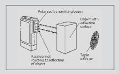
This is a special type of retro-reflective sensor. A special linear or circular polarised filter element (film) is placed between the transmit or receive elements and the glass light emitting face of the sensor.
