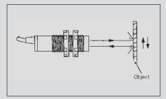
The light transmitter and receiver in a diffuse-reflection sensor are accommodated in one common enclosure. The light emitted from the transmitter is reflected diffused from the detected object. A part of this diffused reflection returns to the receiver and changes the switching status at the output when a certain intensity is exceeded. Accordingly, the texture and the colour of the object surface has a considerable influence on the object detection characteristics (presence – absence).
