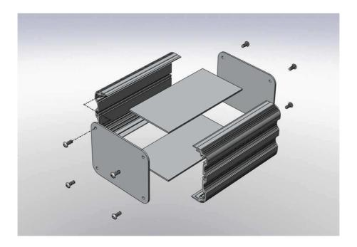
Length Tolerance of extrusion: Nominal length +/-0.3mm e.g. UBES-2-S160 is not shorter than 159.7mm and no longer than 160.3mm.
