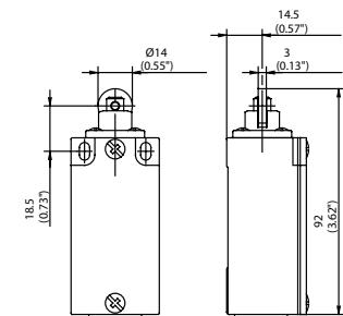
Special features (on request): available for high temperature range and the following contacts: 2 NC / 1 NO; 2 NC / 2 NO (larger enclosure)
