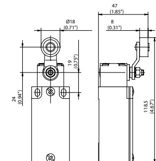
Special feature (on request): available with various roller diameters, cranked or straight lever and with various lever lengths with roller over switch and with the following contacts: 2 NC / 2 NO (larger enclosure)
