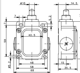
Special feature: Telescopic plunger, particularly long actuation travel of 9 mm
