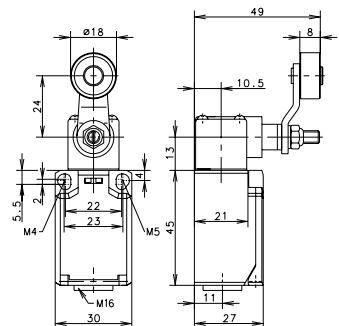
**Special features (on request):** available with different actuating directions; with a steel roller; various roller diameters; cranked or straight lever; various lever lengths; with a roller over switch
